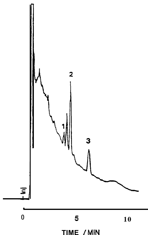
Fig. 14. LC-UV chromatogram of (1) 2,4-dichlorophenoxyacetic acid, (2) 2-methyl-4-chlorophenoxyacetic acid and (3) 2-(2,4-dichlorophenoxy)propionic acid obtained after 24-h field sampling from a brook using an n-undecane-di-n-hexyl ether (1: 1) membrane. Analyte concentrations are about 1 \mu\text{g}/\text{l} . From ref. 56.
